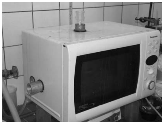
Fig. 3.1 Modified domestic household microwave oven. Inlets for temperature measurement by IR pyrometer (left side) and for attaching reflux condensers (top) are visible. A magnetic stirrer is situated below the instrument.
