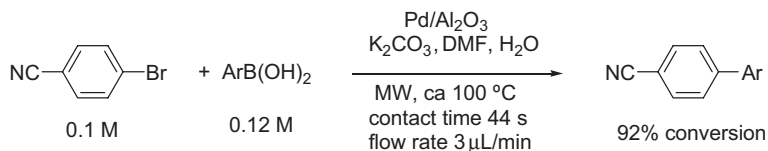
Scheme 4.32 Suzuki reactions in a micro reactor environment.
