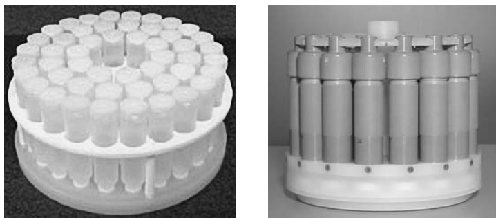
Fig. 3.7 Milestone MultiPREP-50/80 with PFA vessels (left) and PRO 16/24 with PTFE-TFM pressure vessels (right).
