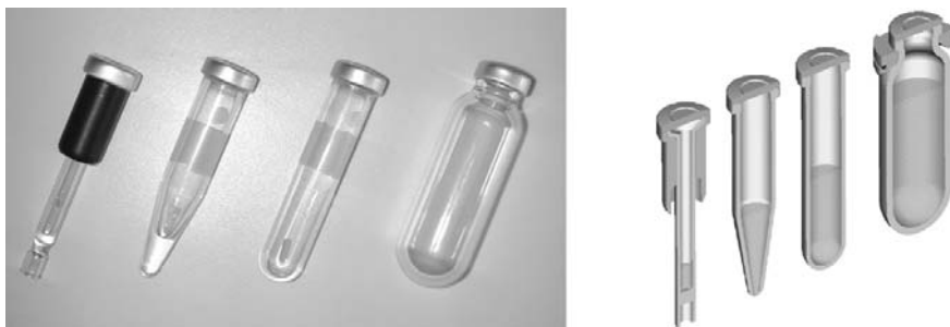
Fig. 3.21 Biotage Initiator vessel types (0.2–0.5 mL, 0.5–2.5 mL, 2.0–5.0 mL, 5.0–20.0 mL (left to right)) and schematic depiction of maximum volume.
