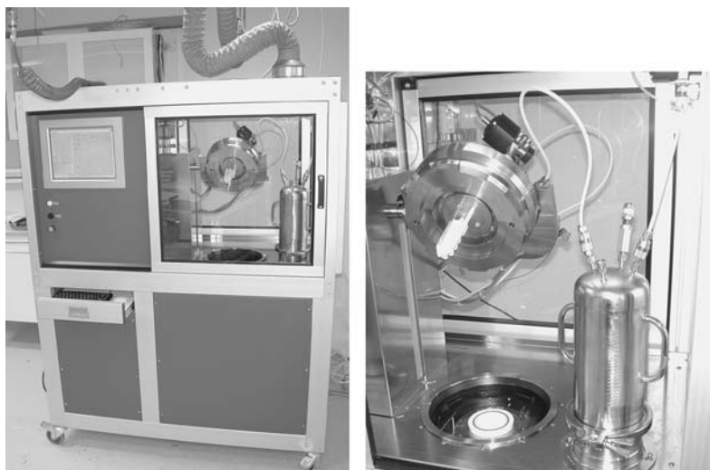
Fig. 3.15 Biotage Emrys Advancer scale-up instrument with multifunctional chamber head (right).
