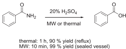
Scheme 1.1 Hydrolysis of benzamide. The first published example (1986) of microwave-assisted organic synthesis.
